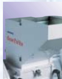
The hopper can be directed in three directions and no-tool detachable.
